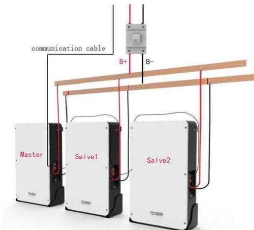
**INV-BAT:** From the master box CAN IN to the inverter CAN port;
