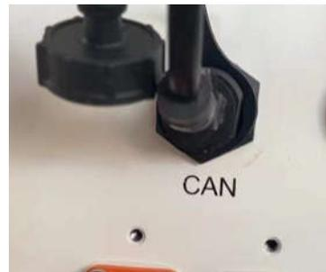
It's normal standard pin-pin cable between battery and inverter ,also battery and battery.
