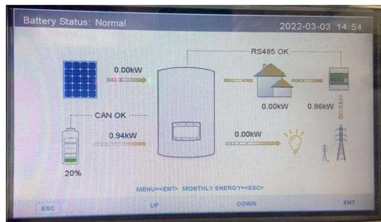
**Step7:**Make the inverter start charging battery to 100% to calibrate SOC.
